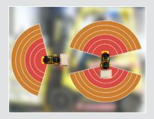
Detection distance of front and rear views can be set between 0.5 to 20 meters.
